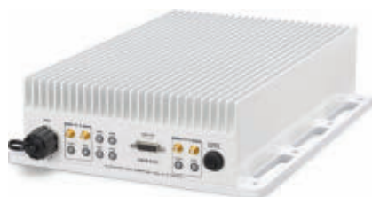
The Pixus Technologies RX310 is a ruggedized version of National Instruments X310 software-defined radio.
