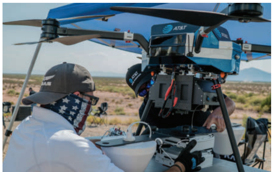
AT&T technicians and civilian contractors assemble a “Cell on Wings” drone to provide 5G connectivity for the Advanced Battle Management Systems Onramp 2 at White Sands Missile Range, N.M.
